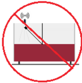
Not Good (Float Interference)
